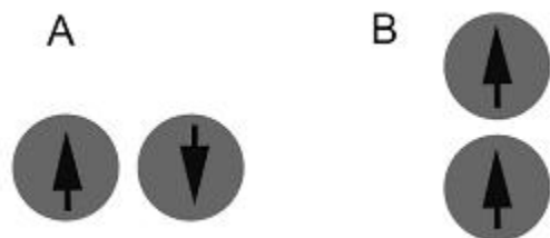
FIG. 12: Energetically favorable orientations of dipoles. (A) Dipoles prefer to align antiparallel when next to each other. (B) Dipoles prefer to align parallel when end to end.
